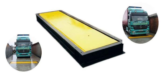
The WB30L axle weighbeam is a robust steel structure supported in each corner by four folded 'S' tensile load cells mounted within specially designed shoes. The platform itself sits in a sturdy steel pit frame, which is set into a flat and level concrete apron (weigh lane).
