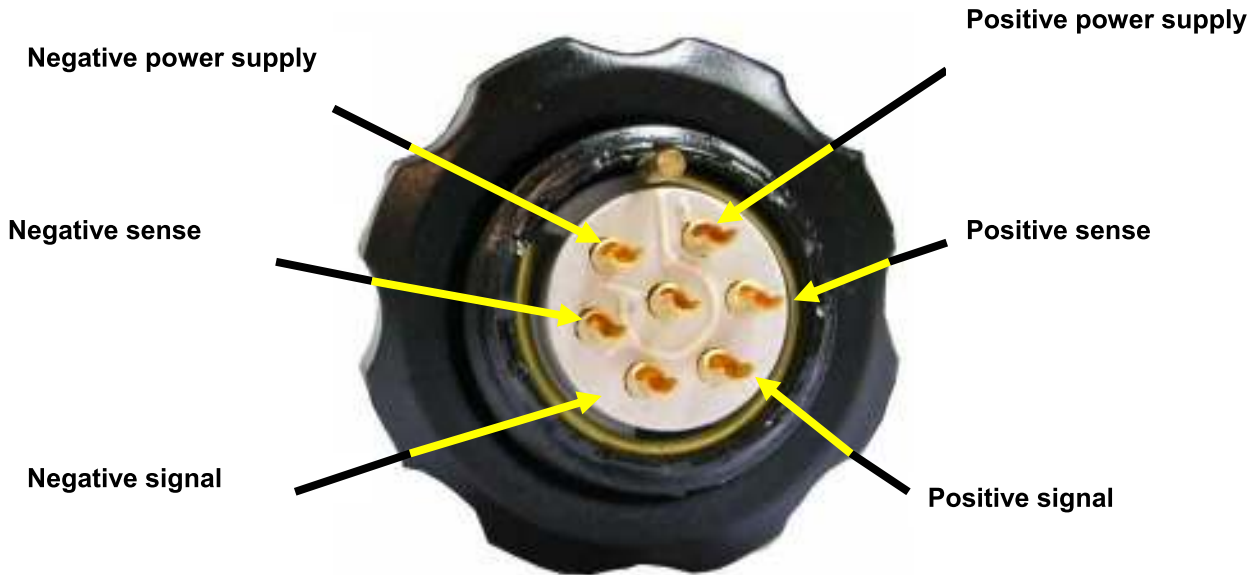
CABLE CONNECTOR (SEEN BY WELDS)
